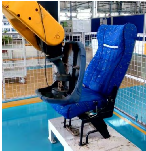
Robotic Ingress Egress test
