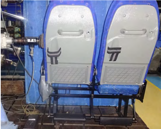
Lateral load test
