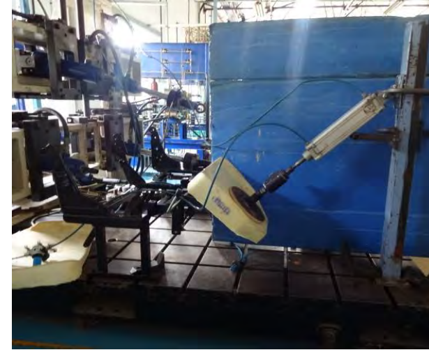
Calf support strength test
