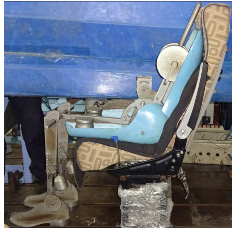
H-Point & Dimension measurement
