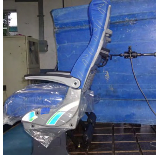
Bottle Holder pull off test
