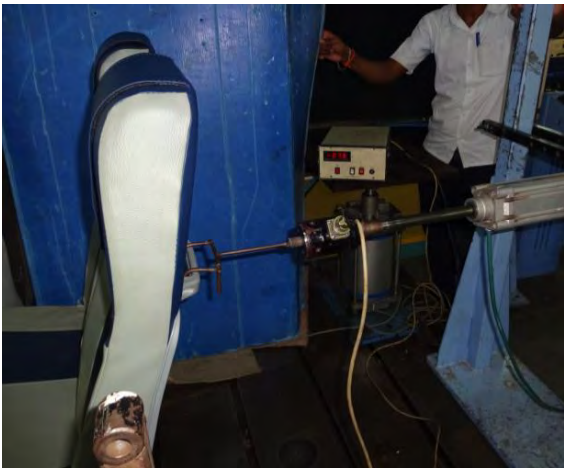
Grab handle pull off test
